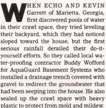
"A homeowner's biggest misconception is thinking that only addressing surface water will stop the leak," Wofford says. "Most basements leak from the ground up where the floor, the footer and the wall meet. As the pressure from underground water increases, it pushes up and through the walls."
